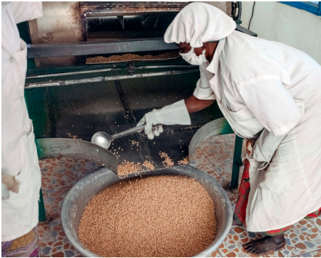
MISOLA staff members lightly toast soybeans over low heat, without burning them to avoid giving the flour a sour taste, February 2021. Photo: Ollivier Girard/Concern Worldwide.
