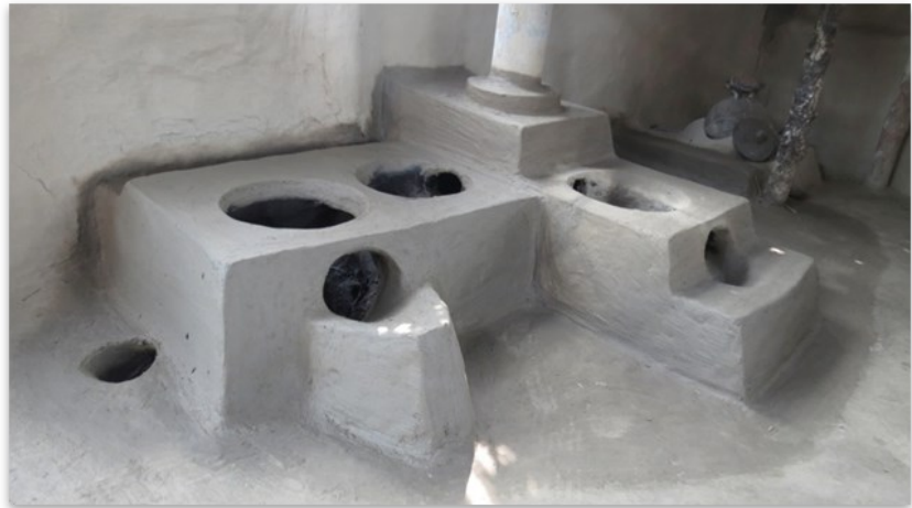
Concern's earth stoves are approximately a third more efficient than traditional earth stoves.
